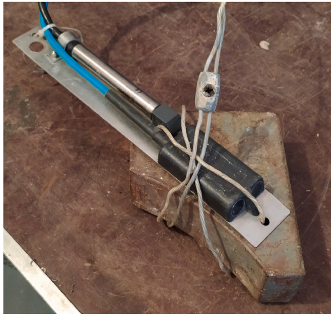
Photo 8. Mainstream 400R probe setup before bottom installation in Section 1. For probe stability deployment at the bottom, an additional weight of 10.5 kg was attached.
