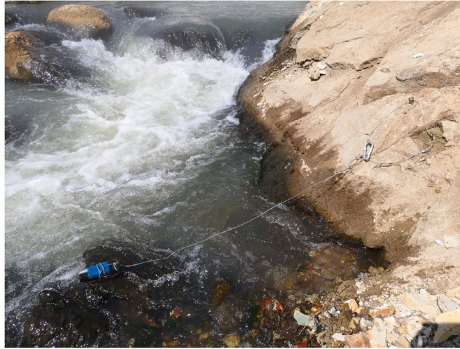
Photo 7. HOBO U20+U24 setup for long-term (month) before bottom installation at section #1 (photo April 21, 2019, Kiryukhin A.V.). Pair of HOBO U20 used for pressure/water level measurements, HOBO U24 was used for specific electro-conductance and temperature measurements.
